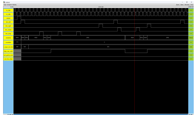
Fig. 14: IRSIM simulation of the core netlist after place and route.
